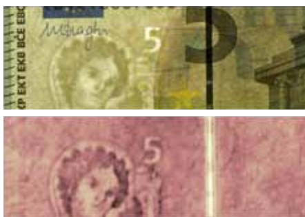
Figure 1: Backlight image and THz image of a watermark
